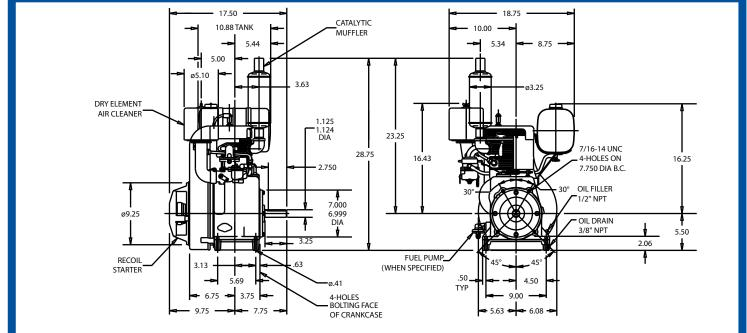
\* Net Weight Dry Standard Engine 110 lbs. (50 kg)
